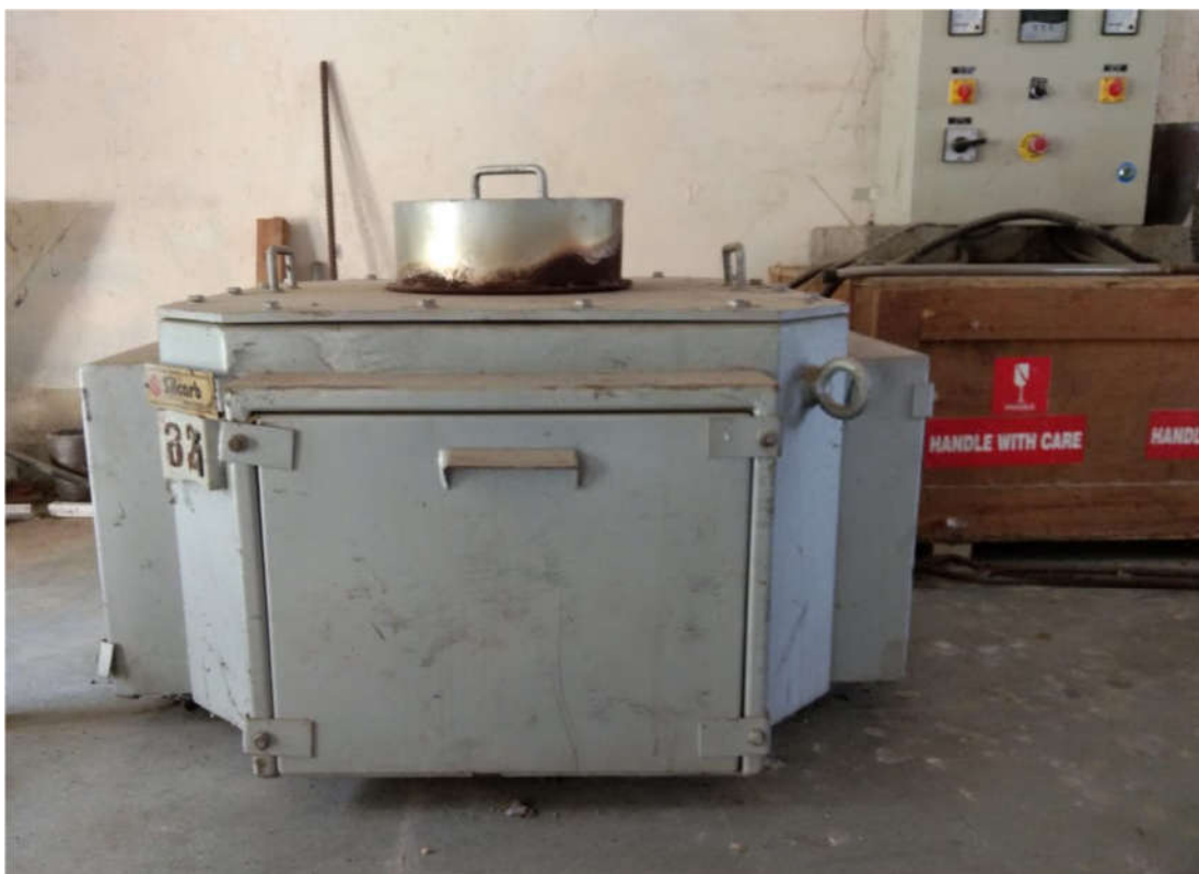
Fig.1 Electric resistance furnace with controll unit.
