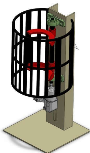
Figure 8: An isometric view of the Spring compressor
