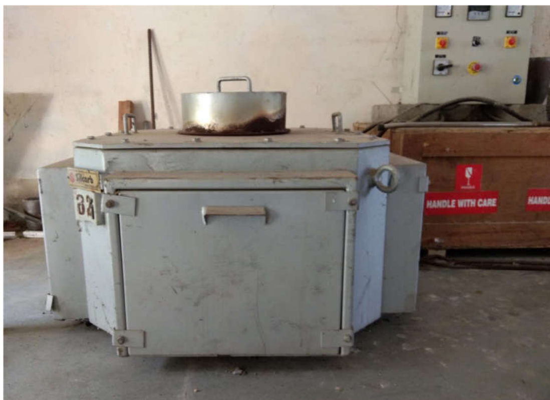
Fig.1 Electric resistance furnace with controll unit.
