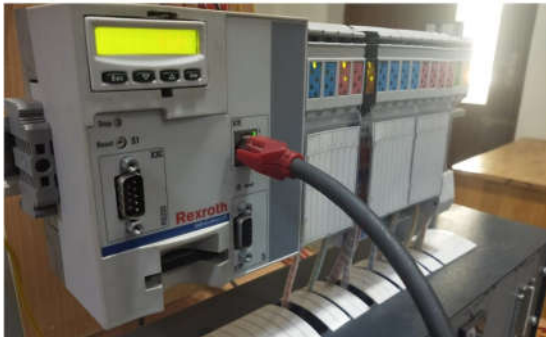
Figure 5: Indra logic kit for PLC
